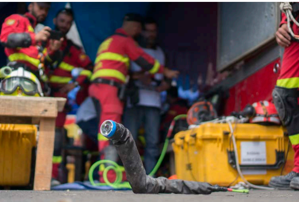
Roboticians and first responders worked together to deploy snake robots after the Mexico City earthquake in 2017.
