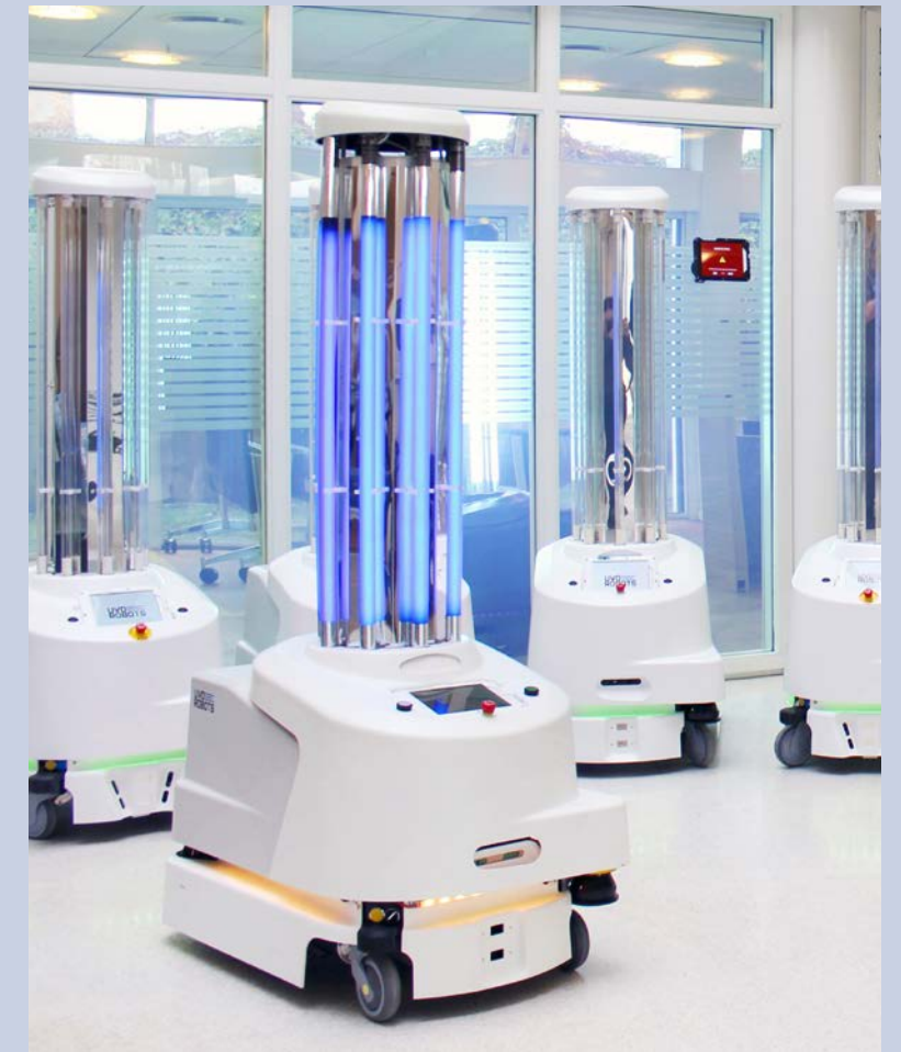
An army of UV-light robots stands at attention; they're already disinfecting hospitals in China and parts of Europe.
